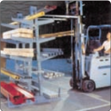
Power trucks can load heavier items on rack with access from either side.
